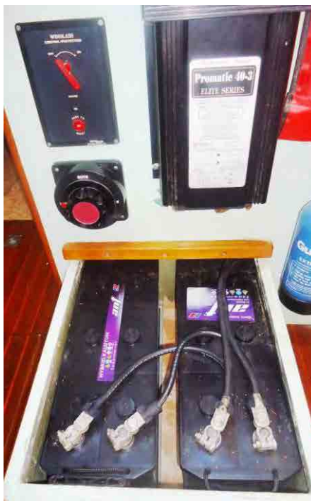
Part Domestic battery bank, selector switch, anchor winch breaker & 220V Battery Charger Kenwood Shortwave Radio – Standard VHF with handset – B & G Depthsounders
